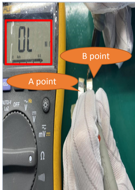
Measure connection of 2 points of FFC led cable
